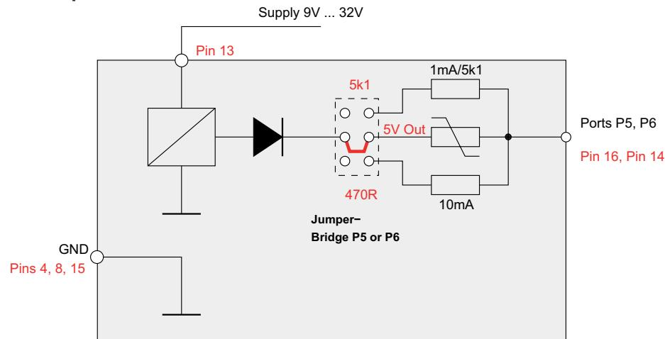
Setting of jumpers for 5 V output: Jumper of P5 and P6 set to contacts in the middle.
