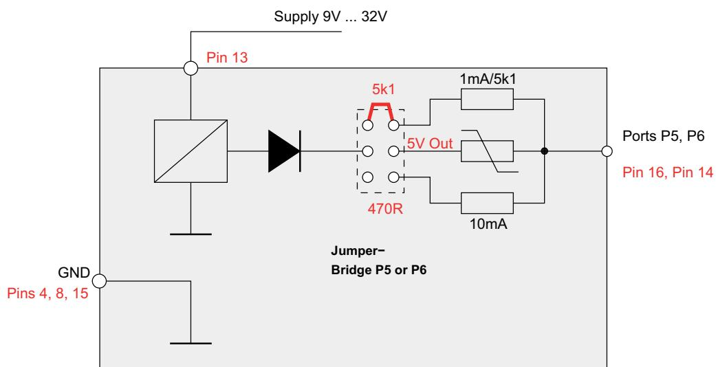
Setting of jumpers for 1 mA output: Jumper of P5 and P6 set to 1 mA (Pull-up 5.1 kΩ).
