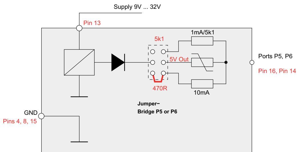
Setting of jumpers for 10 mA output: Jumper of P5 or P6 set to 10 mA.
